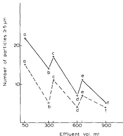
Fig. 6. Contamination recorded with instrumental methods (size ≥ 5 μm) as a function of the effluent volume. Coulter counter (—); HIAC/ROYCO (- - - -).
