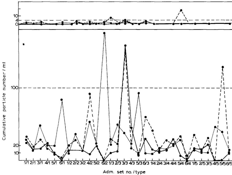
Fig. 1. Analysis of particulate contamination in hemodialysis venous lines. Mean cumulative values/ml for  $\geq 5 \mu\text{m}$ ,  $\geq 10 \mu\text{m}$ ,  $\geq 20 \mu\text{m}$  threshold sizes, determined with the light blockage apparatus. Rinsing sample, (—); sample at  $t = 0$ , (---); sample at  $t = 6 \text{ h}$ , (-·-·-).
