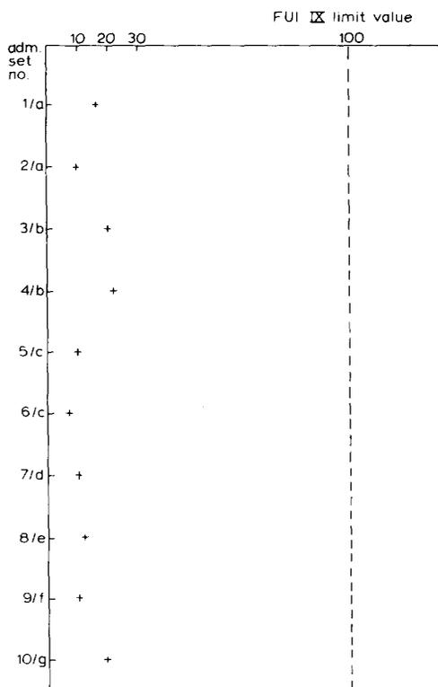
Fig 5. Analysis of particulate matter contamination in phlebotoclysis administration sets. Mean cumulative values/ml for the 5 μm threshold size, as determined with the light blockage apparatus.
